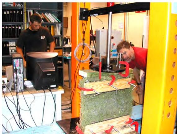
Fig. 2. Hydraulic apparatus with load cell was used to measure sod tensile strength.
