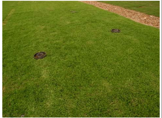
Figure 3. Measurement of infiltration rates using double-ring infiltrometers.
